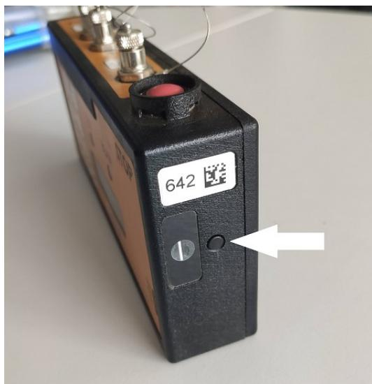
Once the button is in OFF position, the clock, the modem and the beam Led will not work.
